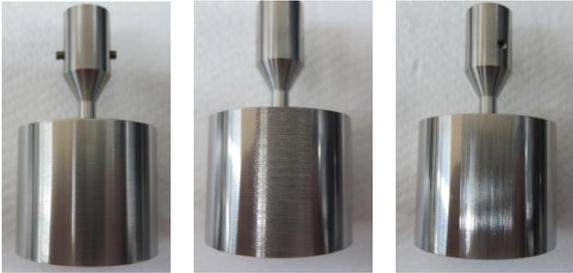
Fig.3 (a) Non-groove inner cylinder (b) Transverse groove inner cylinder (c) Longitudinal groove inner cylinder
