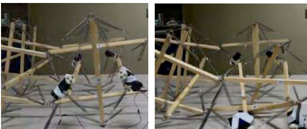
Fig.4 Elastic body winding with tensegrity
