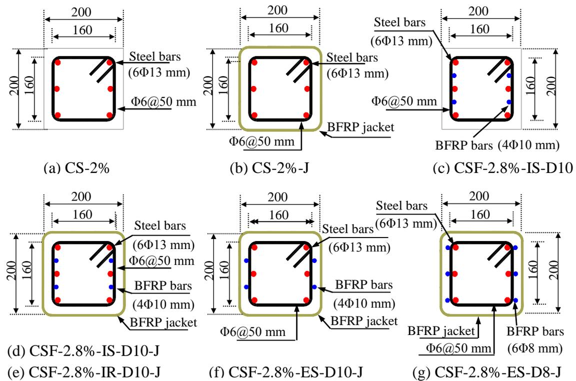
**Fig. 4.** Cross sections and reinforcement details of specimens (dimensions are in mm)
