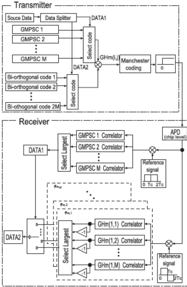
Fig. 2 System structure of CSK with the new PN code.
