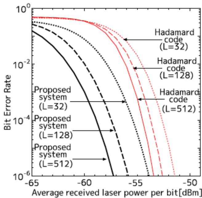
Fig.4 BER versus average received laser power per bit, where  $L = 32, 128$  and  $512$ .
