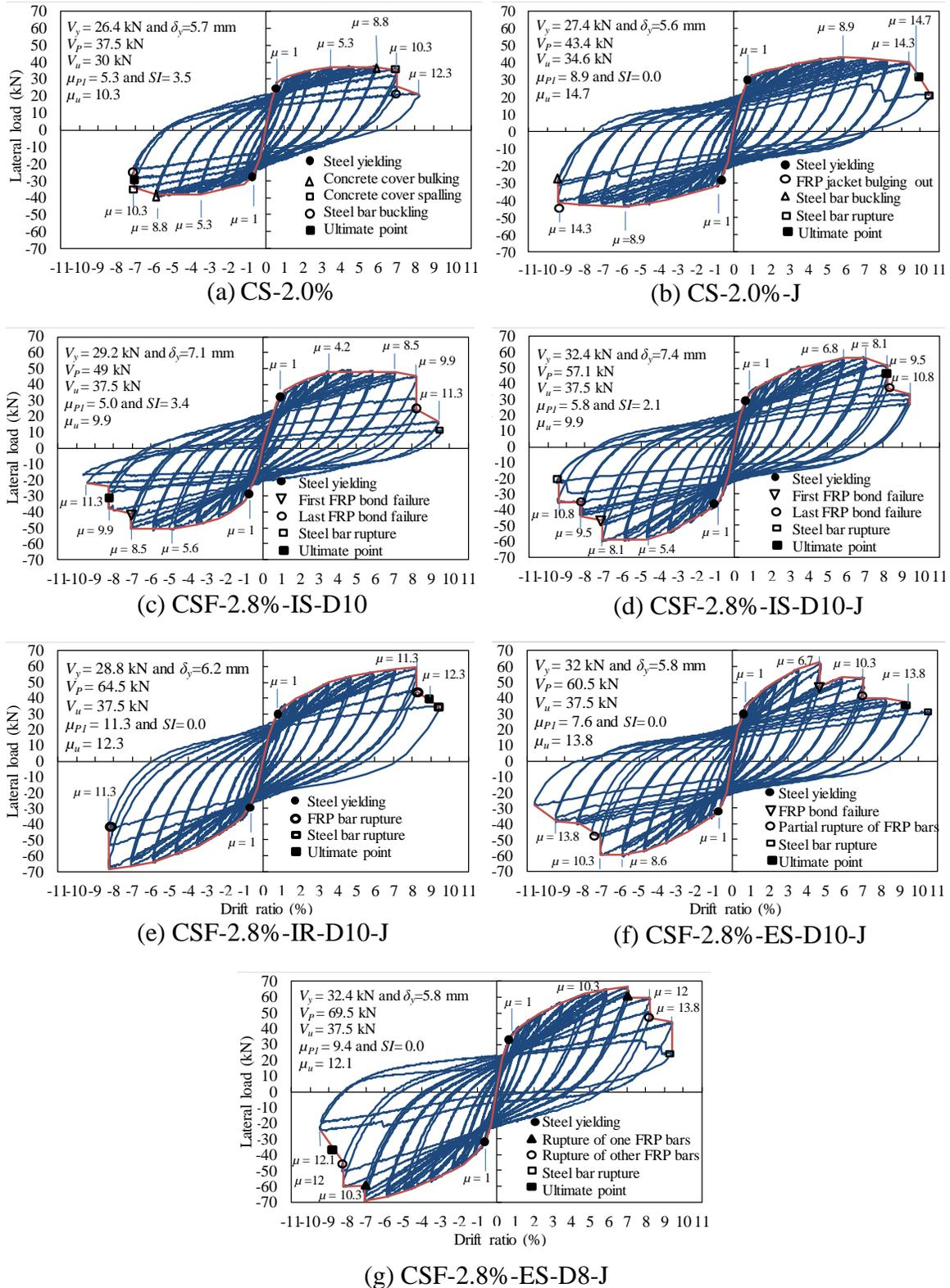
Fig. 7. Load versus drift ratio curves of column specimens
