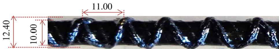
(c) 10-mm-diameter BFRP bar with cross roughened surface (rough D10 bar)
