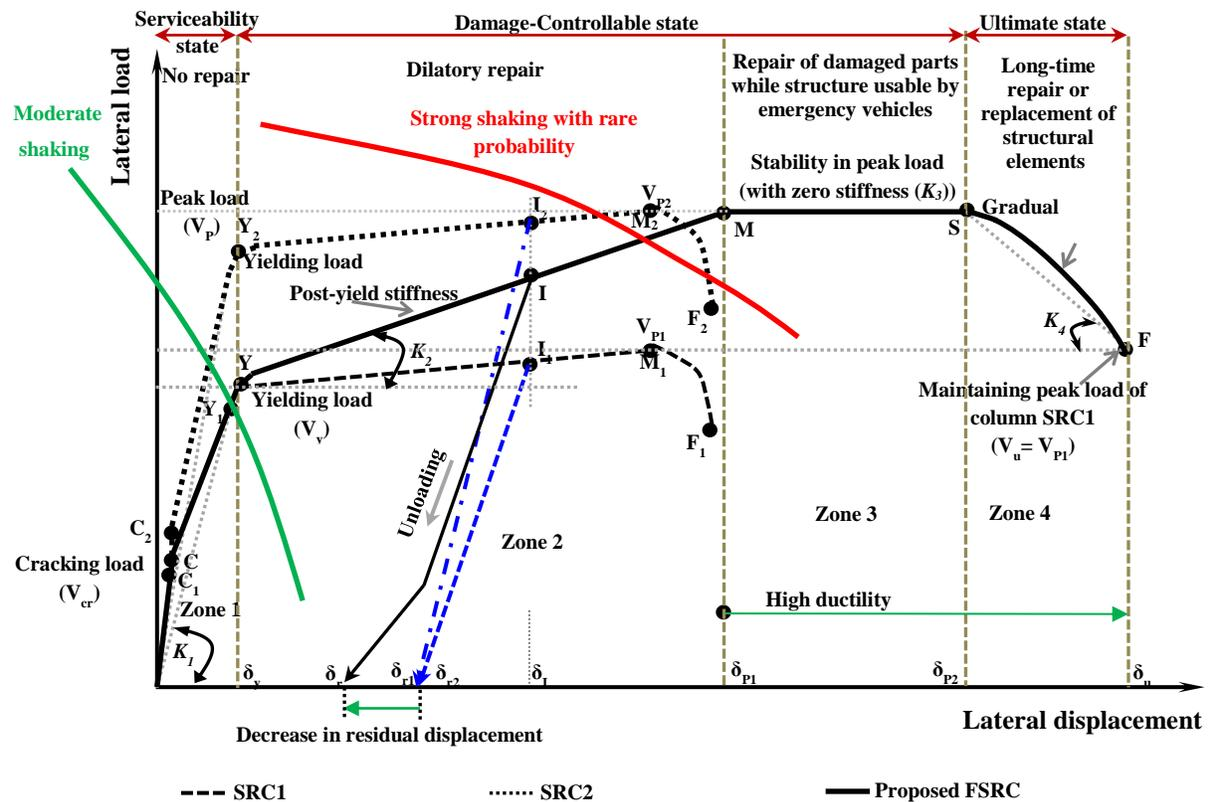
**Fig. 2.** Targeted idealized load deformation behavior of the proposed FRP-steel RC column versus steel RC columns, based on the damage-controlled model for existing RC structures
