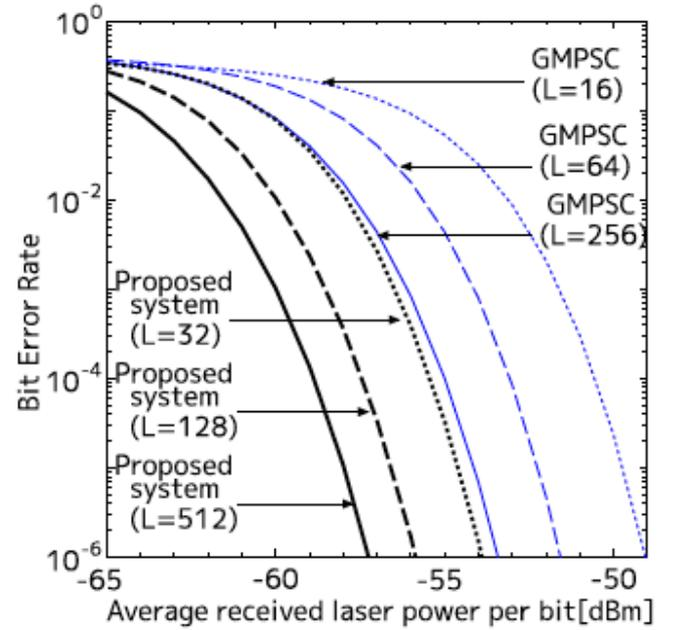
Fig. 3 BER versus average received laser power per bit, where  $L = 16, 32, 64, 128, 256$  and  $512$ .
