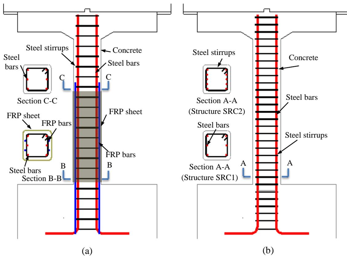
**Fig. 1.** Schematic model of: a) proposed FSRC structure and b) conventional SRC structure (SRC1 and SRC2)
