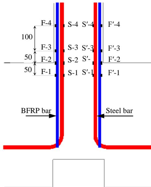
**Fig. 6.** Typical arrangement of strain gauges
