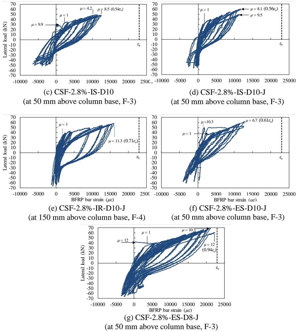
**Fig. 9.** Load versus BFRP bar strain of FSRC columns
