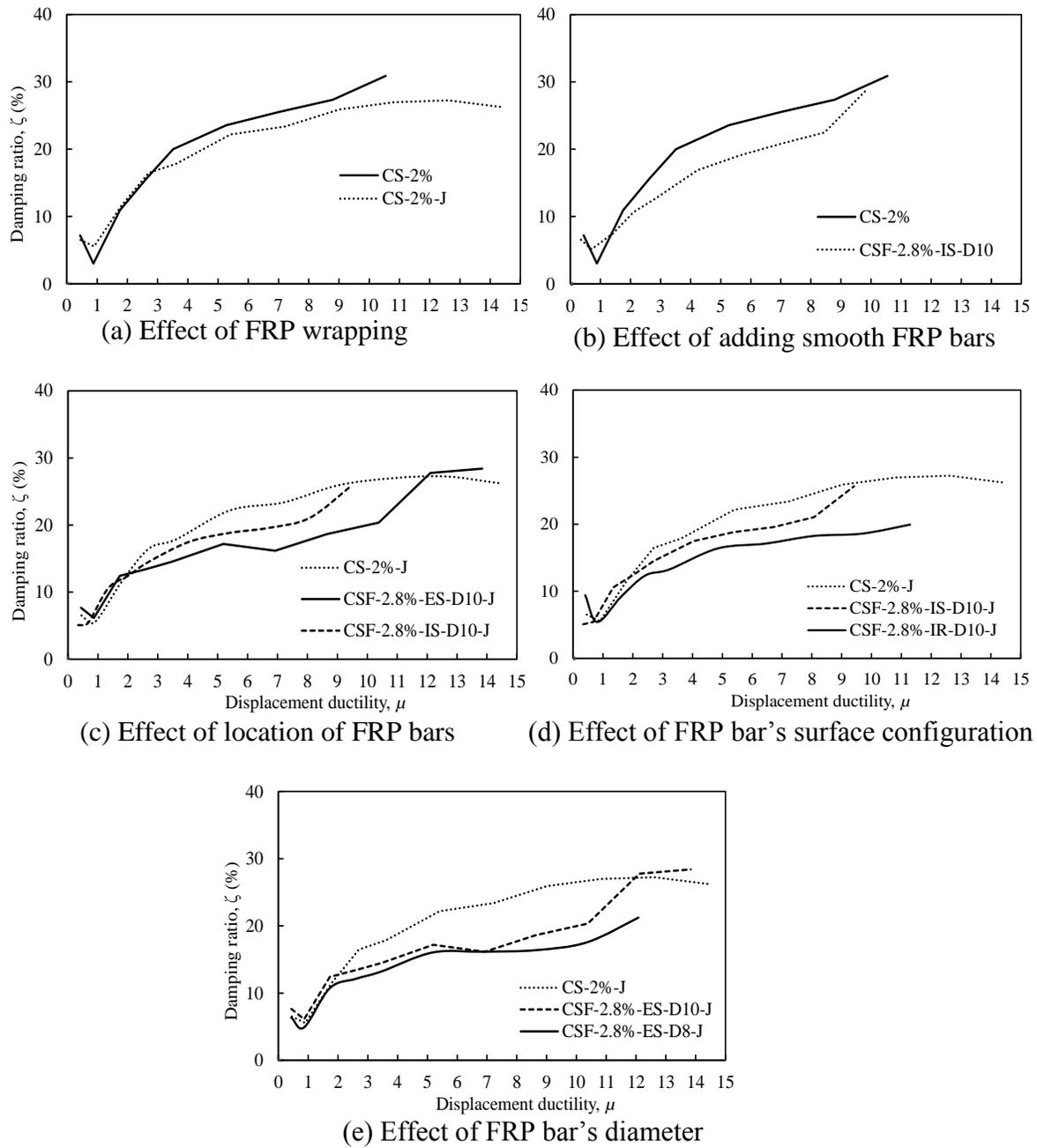
**Fig. 13.** Effect of all investigated parameters on the damping ratio
