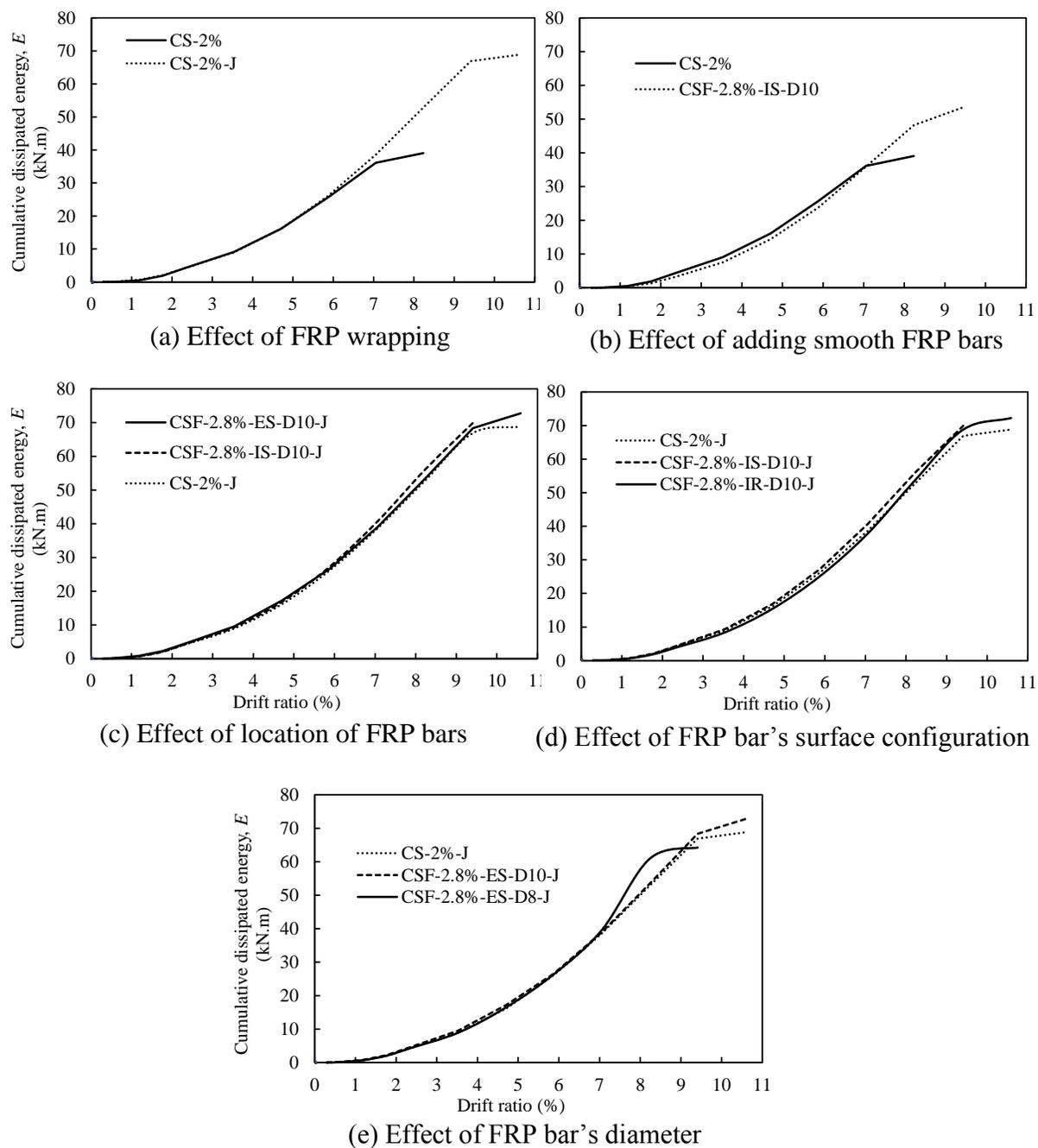
**Fig. 12.** Effect of all investigated parameters on the cumulative dissipated energy
