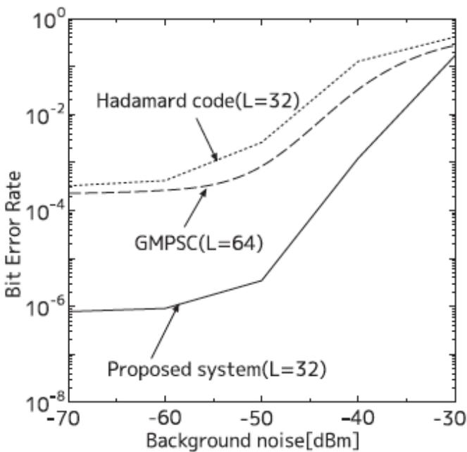
Fig.5 BER versus Background noise ( $P_b$ ) when average received laser power per bit ( $P_{bit}$ ) =  $-55$  [dBm], and  $L = 32$  and  $64$ .
